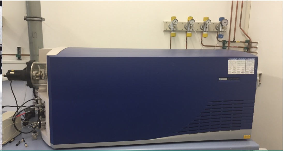
Waters Quattro LC, 2000, first LC-MS/MS system in the LMU-Lab
