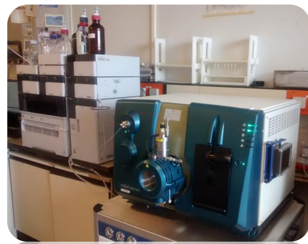
Figure 1. LC-MS/MS system used for E1/E2 determination
