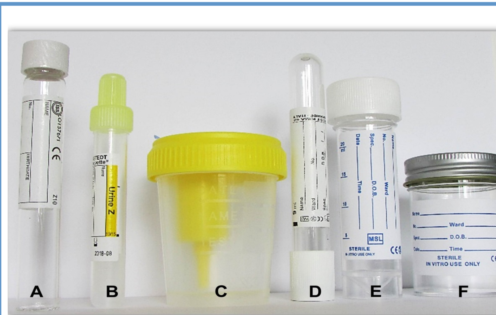
Figure 1. A photograph of the urine sample containers investigated in this study. A: glass; B: monovette; C: vacutest 60 mL; D: vacutest 9 mL; E: universal; F: metal cap.
