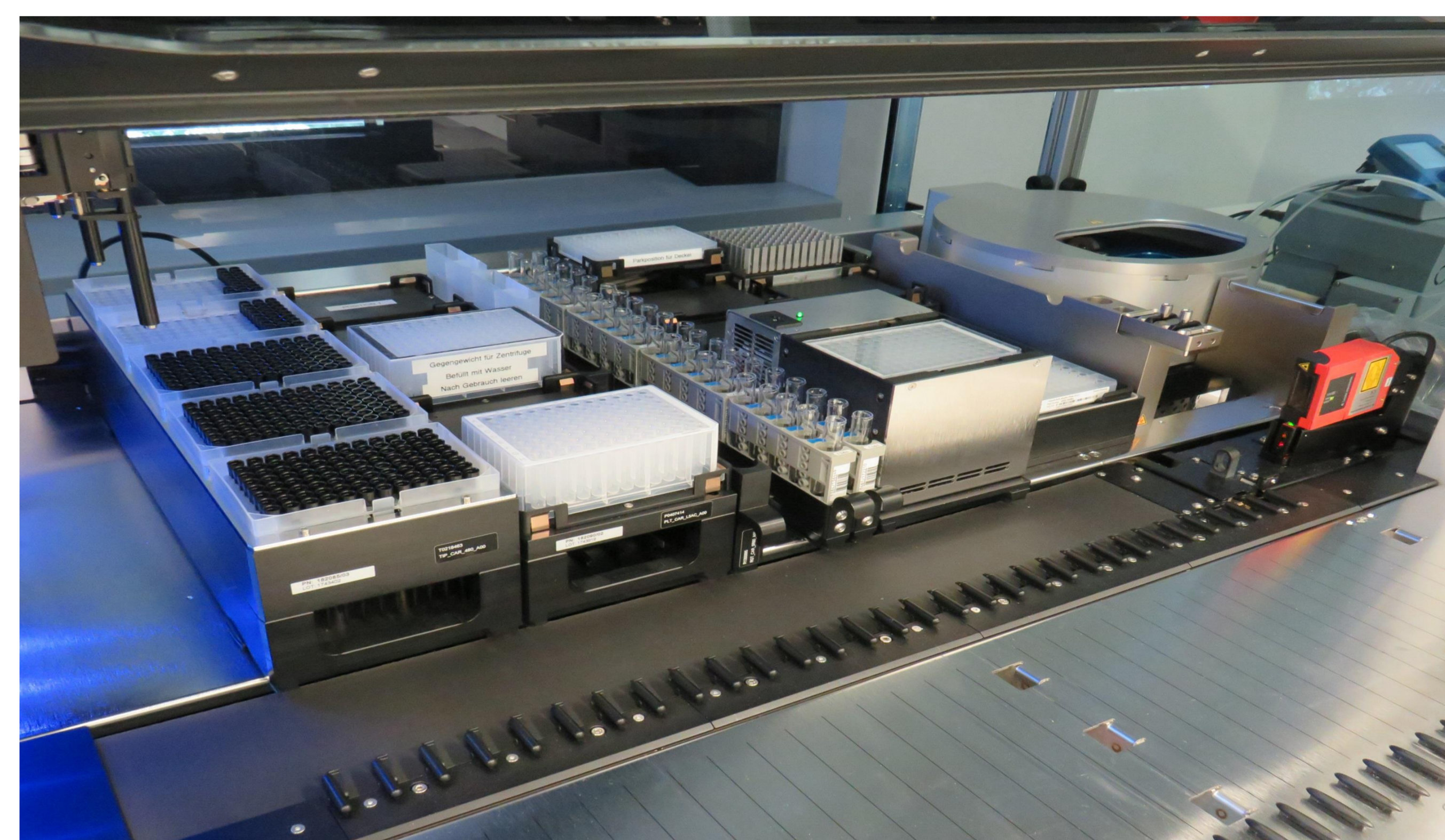
Figure 1: ML STARlet equipped with a centrifuge, vacuum station, heater shaker and cooling module; further available methods are immunosuppressant, neuroleptics, antiepileptics, antidepressants and antibiotics;
