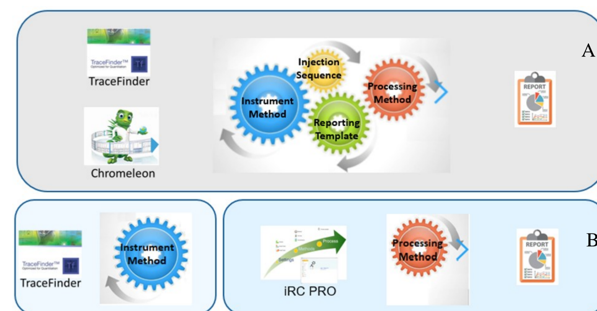
Figure 5. Workflow comparison between TraceFinder, Chromeleon and iRC Pro SW. A) Both TraceFinder and Chromeleon SW can use one software platform for data acquisition, processing, and reporting. When instrument method, processing method, reporting template and injection sequence are defined and ready, one click will initiate sample sequence submission with automated reporting. The strategy can provide a single, complete audit trail for acquisition, processing, and reporting, which would reduce and simplify audit preparation. B) iRC PRO SW has simple user interface. It can process raw data to reports, with behind-the-scene built-in peak integration, calculation method, and reporting template. Setting up of the automated data processing can be started without learning the details of TraceFinder SW.
