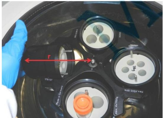
$$G = (1.118 \times 10^{-5}) \times r \times (\text{RPM})^2$$
